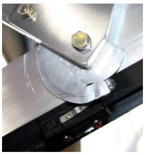
angle is exceeded. One way of achieving this is to fabricate a cam that continuously closes a switch whenever the flaps exceed a predetermined angle.
